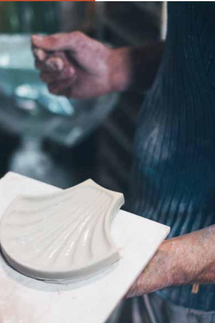
In the production process of Artigiana, the creation of each tile is followed individually by our craftsmen. After having cut to size the mixed base of raw materials and pressed it, the raw biscuit goes in the drying phase for one week then it goes in a traditional muffle furnace that slowly fires the biscuit for 18 hours at 1000 C.
